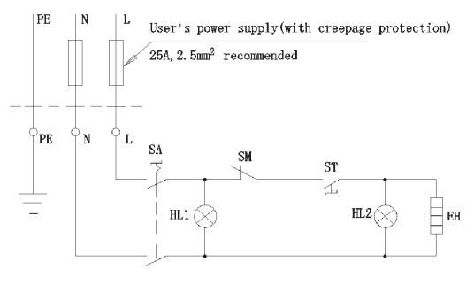
SA:Main Switch SM:Limiter ST: Temperature contoler
