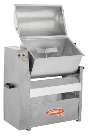
Following the meat processing market growth Fleetwood by Skymsen's 100 lbs capacity Meat Mixer meets the needs of small to medium sized sausage and hamburger making clients. Stainless steel tilting bowl, shafts and blades. Safety bowl cover cuts power when raised or tilted. Pulse switch activates mixer when tilted for ease of unloading.
