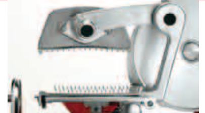
Lateral movement with a clamping arm to slide product through
