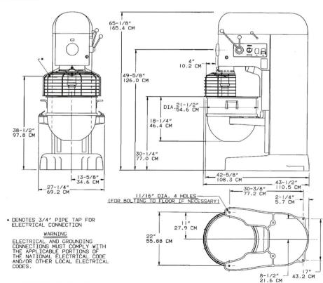
BOLTING TO FLOOR UNNECESSARY EXCEPT ON SHIPBOARD
