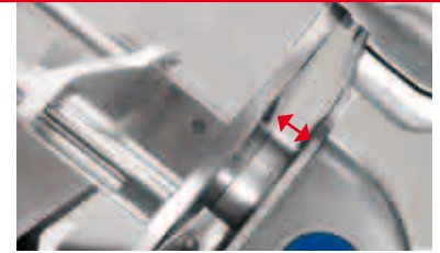
Increased gap between blade and machine body
